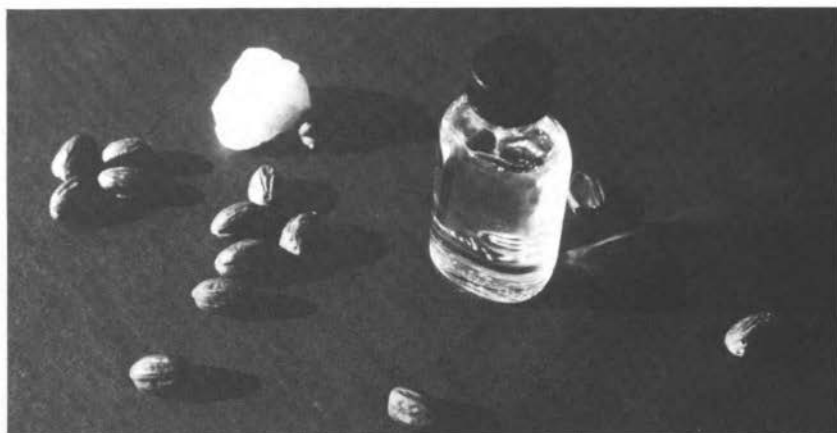
Jojoba seeds, oil, and the very hard wax that is obtained by hydrogenating jojoba oil. (E. Battaglia)
