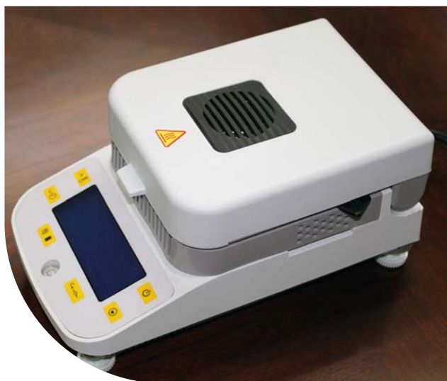
Moisture analyzer that uses heat to achieve a constant dry weight.
