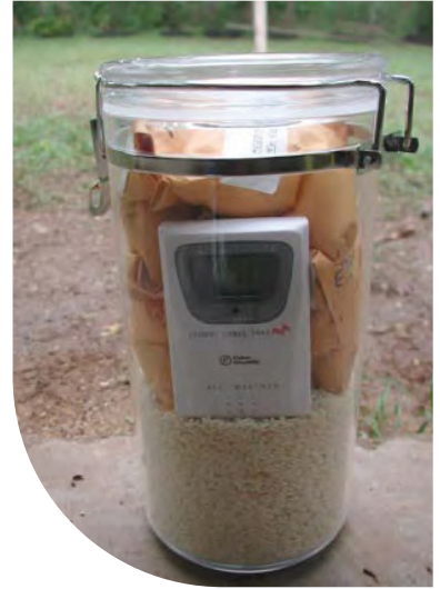
Rice as a desiccant placed in the bottom of a sealed container with envelopes of seed placed over the rice. Note the wireless hygrometer used to monitor humidity.
