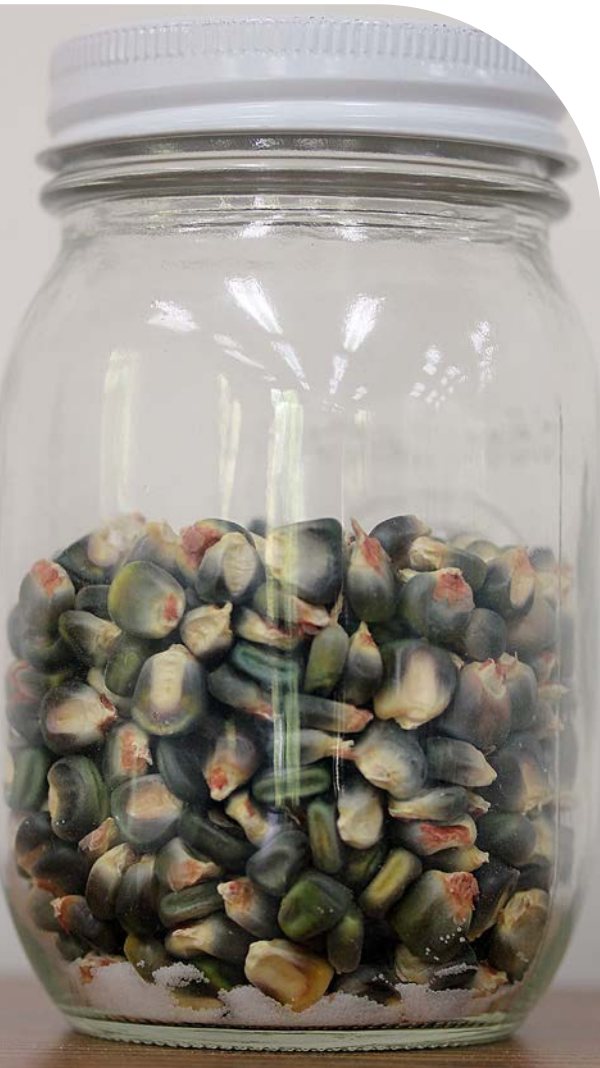
Salt jars with subsamples of maize seed; salt at bottom of jar indicates dry seed.
