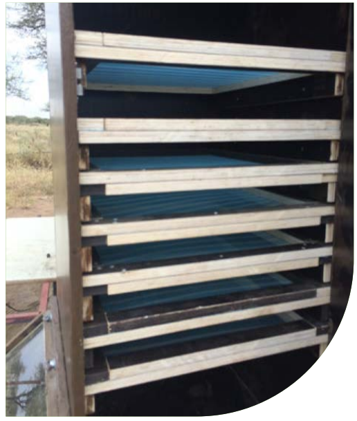
Chimney solar drier for drying plant biomass or seeds.
