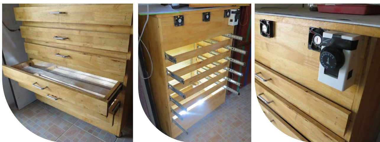
Seed cabinet dryer equipped with drawers (left), hardware for removable screen shelves (middle), light bulbs as the source of heat (middle), thermostat for temperature control (right), and DC computer fans for air circulation (right).
