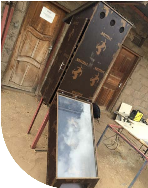
Chimney solar drier for drying plant biomass or seeds.
