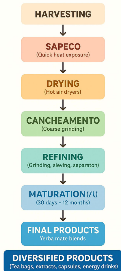
FIGURE 1 | Flowchart of the industrial processing chain of Ilex paraguariensis and its influence on product quality.
