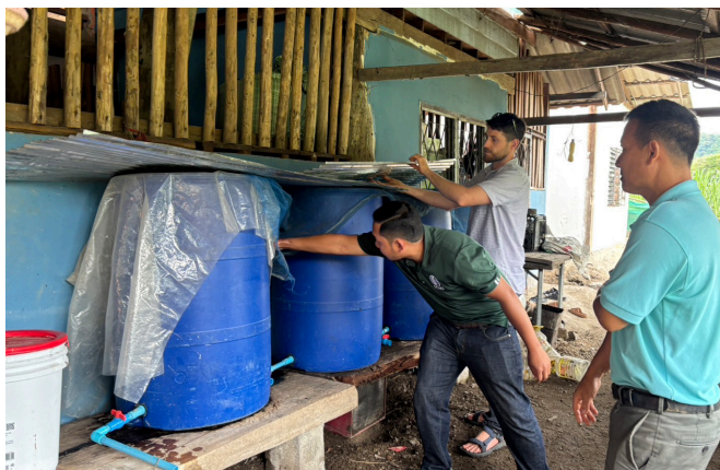
Figure 10. Checking a biosand water filter and taking water samples in Pangfan village. Source: ECHO Asia Staff
