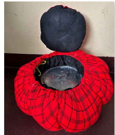
Figure 4. A cloth-covered fireless cooker with a pot and lid. Source: ECHO East Africa staff
