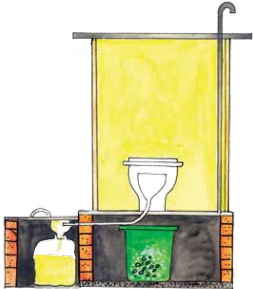
Single chamber, sitting, attached wipers with urine collection. (Reference: Ecological Sanitation- Revised and Enlarged Edition , Stockholm Environment Institute 2004)
