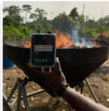
Figure 2. A Kon-Tiki kiln (left) and dMRV process in Ghana (right). The image on the right shows the Greenbox device from Planboo, a thermal IoT sensor installed on each kiln to monitor the pyrolysis process. Source: Samuel Gyasi
