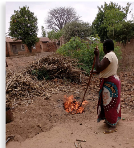
Figure 5. Biochar Life biochar supplier using a simple trench kiln in Malawi. Source: Warm Heart Worldwide
