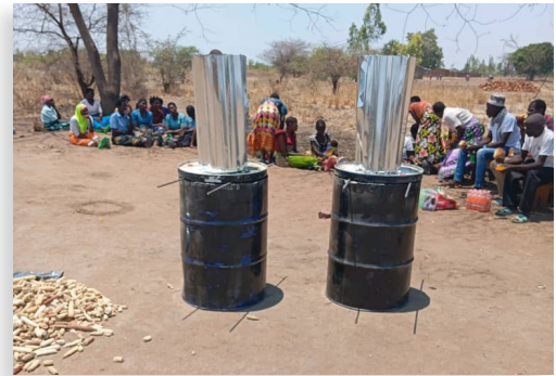
Figure 4. Warm Heart biochar training with Top Lit Updraft Kilns in Malawi. Source: Warm Heart Worldwide
