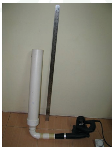
Figure 8. Method of drying seeds inside a PVC column using an air blower (left). Screens are shown (below), which hold the seeds in place within the PVC column.
