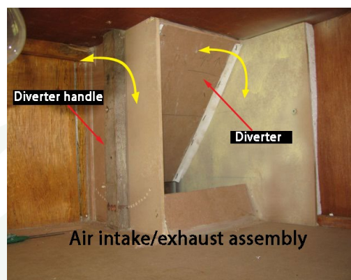
Figure 7. Seed dryer cabinet (left) and diverter assembly (right) modified for use where it is necessary to exhaust humidity in the cabinet
