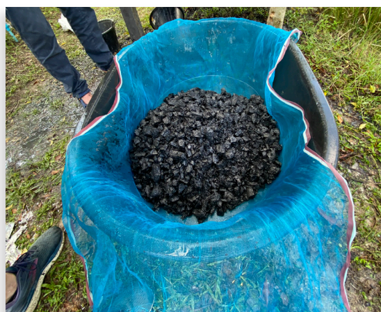
Figure 9. Wrapping char in mesh bag ready for installation. Source: ECHO Asia
