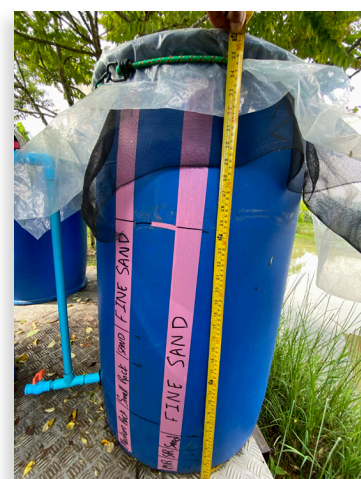
Figure 5. Recording specifications of the thickness of layers of different particle sizes. Source: ECHO Asia
