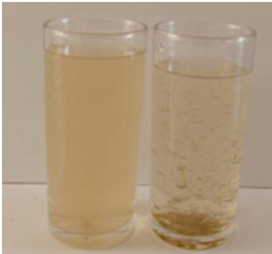
Figure 6. Before (left) and after (right) filtration with the first design. Source: ECHO Asia
