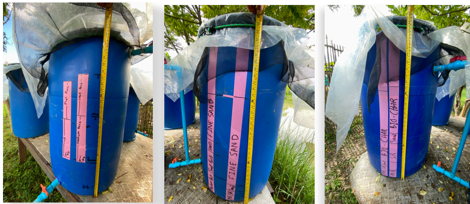
Figure 12. Pink strip showing round 1 and round 2 material depths for the first (left/gravel), second (middle/sand), and third (right/char) barrels. Source: ECHO Asia
