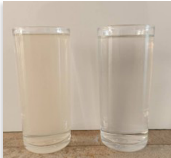
Figure 7. Before (left) and after (right) filtration with the modified design. Source: ECHO Asia
