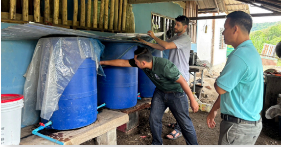
Figure 3. Checking a bio-sand water filter and taking water samples in Pangfan village. Source: ECHO Asia
