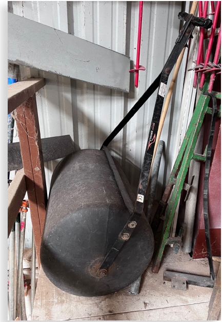
Figure 2. Simple water roller to help increase seed-to-soil contact in coarse soils. Source: Tim Motis
