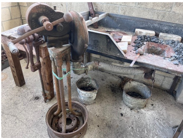
Figure 18. Forge used at ECHO to heat beads made with clay and wood ash. Source: Tim Motis
